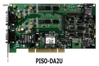
Universal PCI, 2-ch Isolated Analog Output Board
